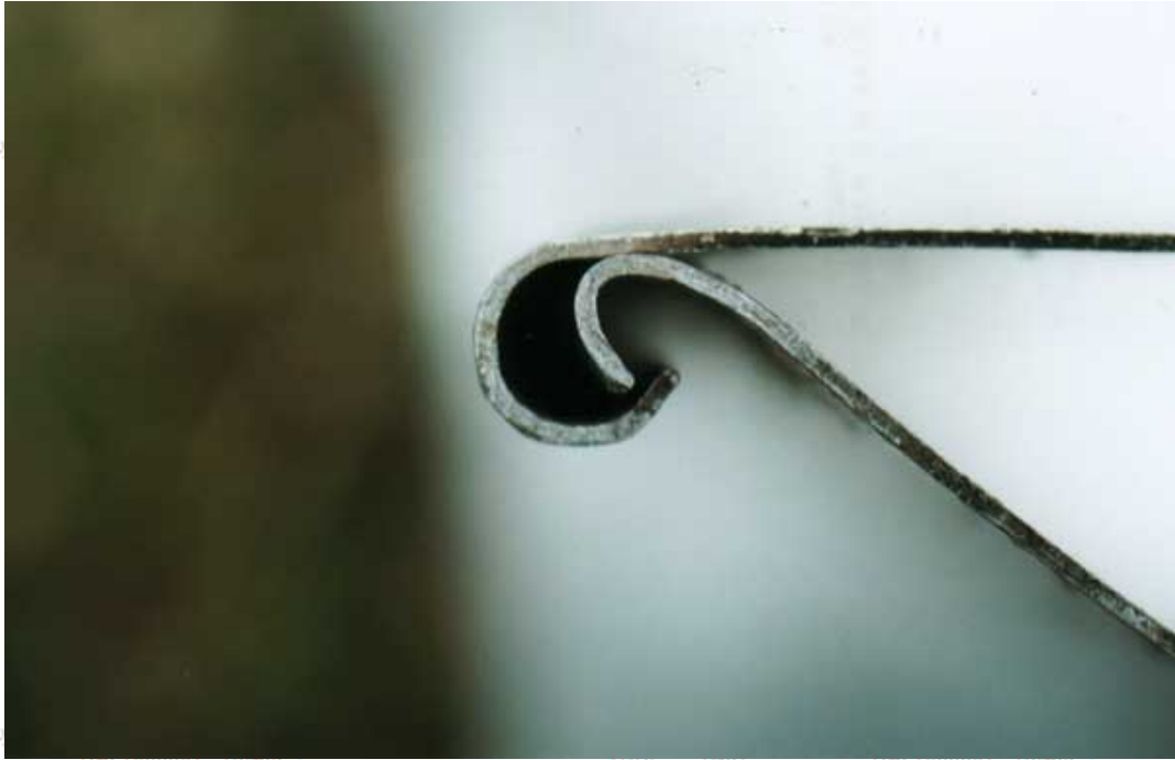
This photo illustrates the bend where the cooking plate joins the bottom plate.
